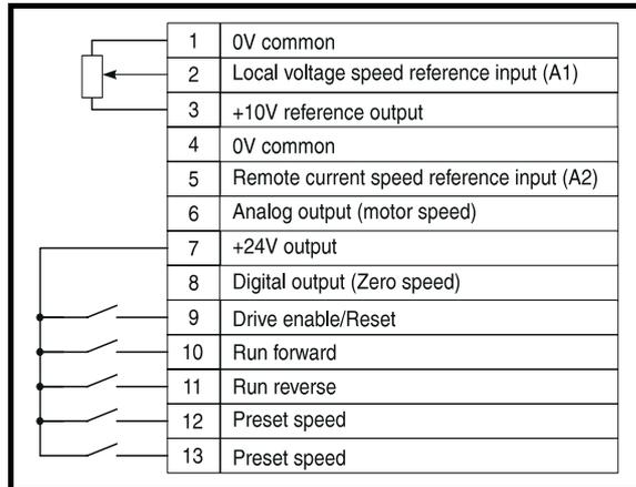
**Figure 6.4 Terminal connections**
