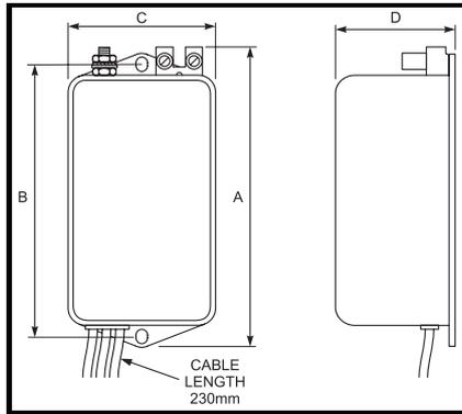
**Figure 4.3 Size 1 Low cost filter dimensions**
