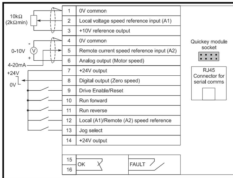
Figure 5.3 Control terminal connections
