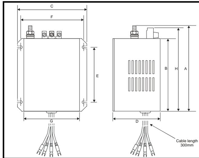
**Figure 4.5 RFI Filter Dimensions**
