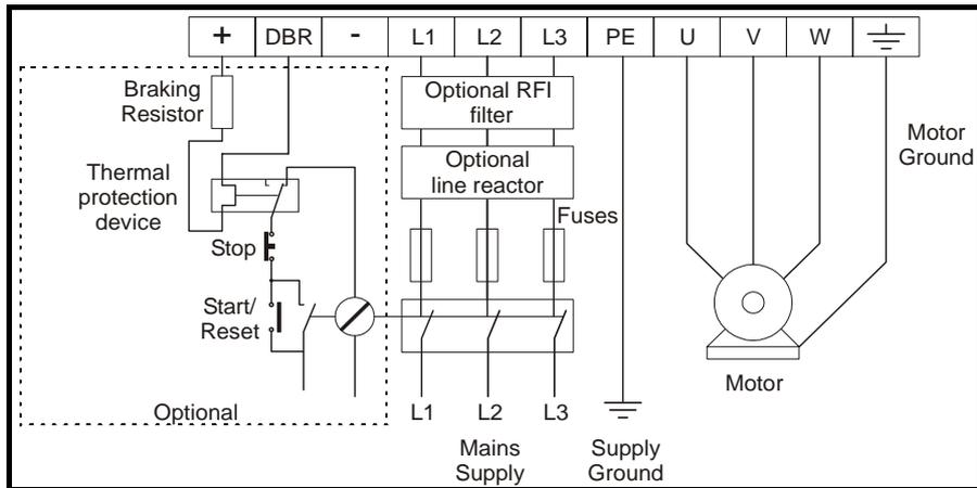
Figure 5.2 Commander SE Size 2 to 4 power terminal connections
