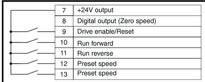
**Figure 6.6 Terminal connections**
