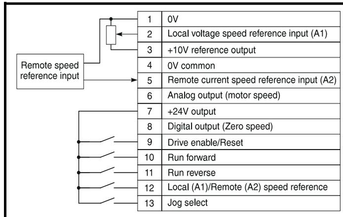
**Figure 6.3 Terminal connections**
