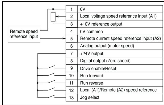
**Figure 6.3 Terminal connections**
