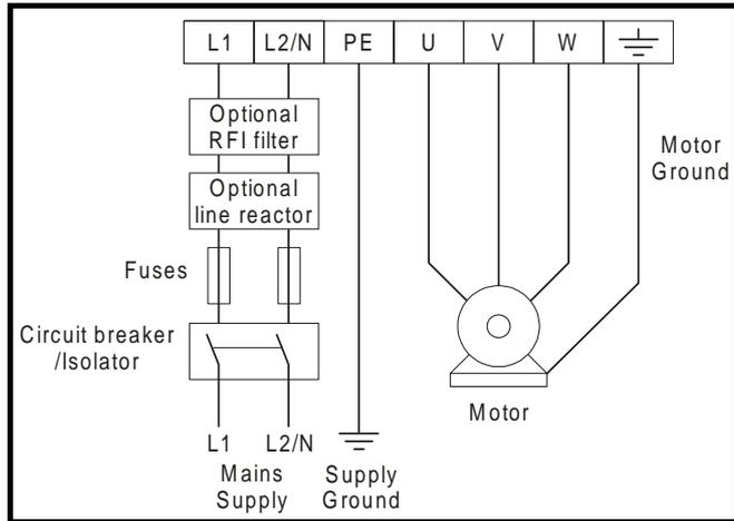
Figure 5.1 Commander SE Size 1 power terminal connections
