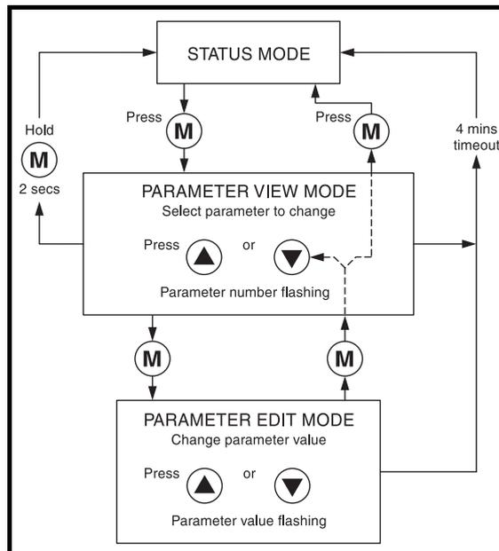
Figure 6.2 Selecting and changing parameters
