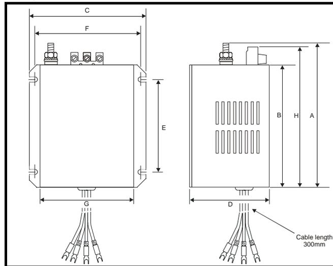
**Figure 4.5 RFI Filter Dimensions**
