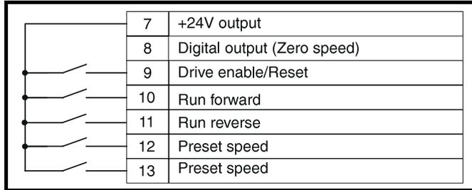
**Figure 6.6 Terminal connections**
